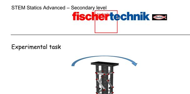
While the structure frame can still absorb vertical and horizontal forces, the spiral-shaped arrangement makes torsion possible; if you hold the tower at the bottom and twist the top plate around its centre you will see that the structure of the tower yields under this load. This does not usually present a problem for a real tower, since stress of this kind is not likely to occur on a tower.
