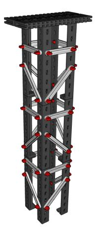
Now test which of the faults you observed have been eliminated by bracing using the structural struts.
