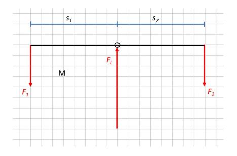
4. Calculate the moments around the fulcrum which result from individual weights and form the sum. When is the lever in equilibrium mathematically? What would that mean for the length of the lever if the weight were doubled on one side?
